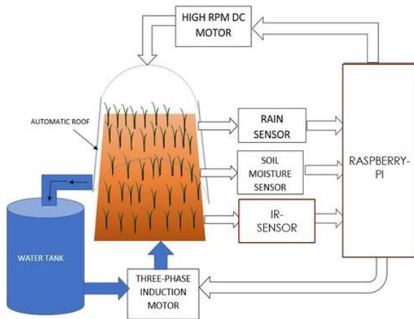
Fig 1: Block Diagram of the Proposed System
