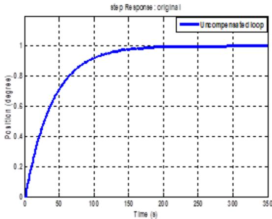
Fig. 4 Step response performance for uncompensated system
