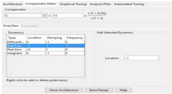
Fig. A3 GUI of the designed compensator
