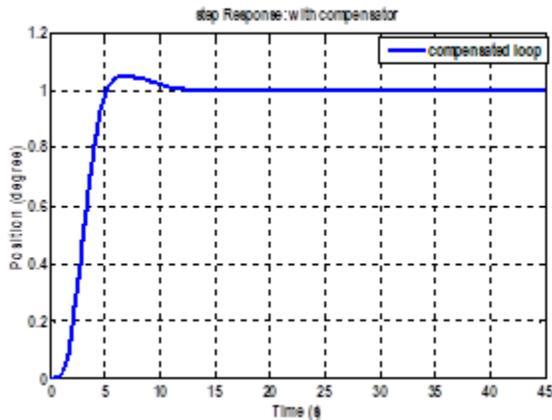
Fig. 5 Step response performance for compensated system
