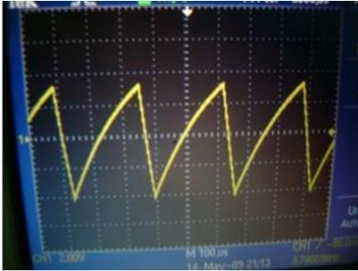
Fig. 7.0: Triangular waveform
