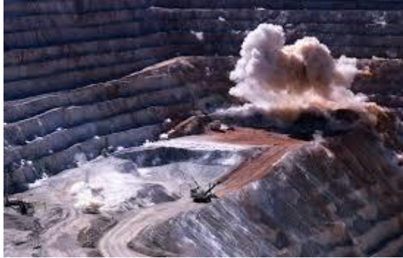
Fig-4 Blasting in O/c mines [12]
