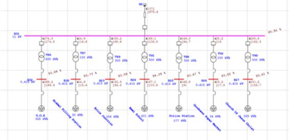
Fig. 5, Iwofe 3Distribution Network before Application of Optimization Network
