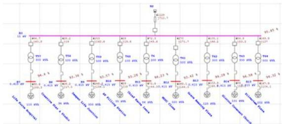
Fig. 3, Iwofe 1 Distribution Network before Application of Optimization Network
