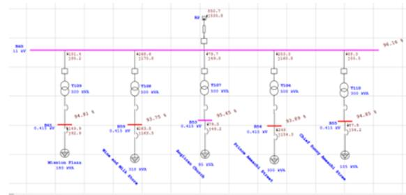
Fig. 7, Aker Road Distribution Network before Application of Optimization Network
