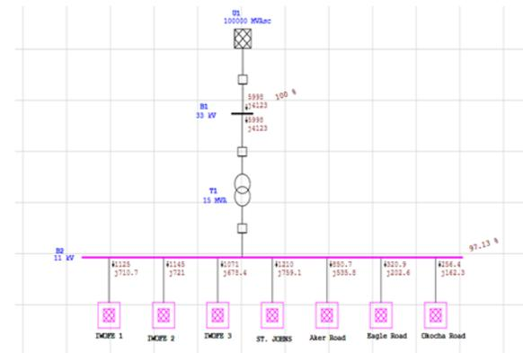
Fig. 2, Iwofe Injection Substation before Application of Optimization Technique
