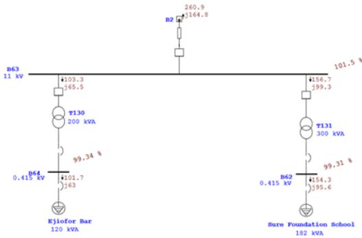
Fig.16 Okocha Road Distribution Network after Application of Optimization Network
