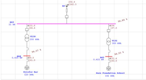
Fig. 8, Okocha Road Distribution Network before Application of Optimization Network
