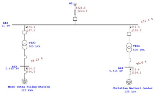
Fig.17 Eagle Road Distribution Network after Application of Optimization Network
