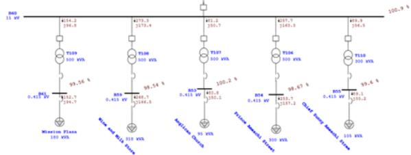
Fig.15, Aker Road Distribution Network after Application of Optimization Network
