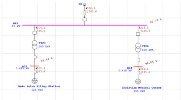
Fig. 9, Eagle Road Distribution Network before Application of Optimization Network
