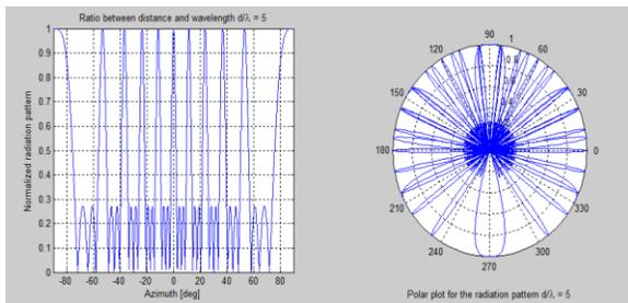
Figure 5: Plot of radiation pattern with 4 element array and separation distance  $5\lambda$
