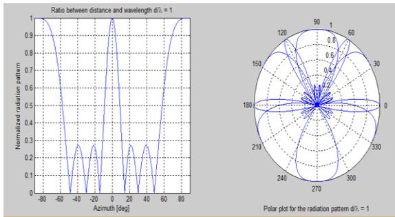
Figure 3: Plot of radiation pattern with 4 element array and separation distance  $1\lambda$
