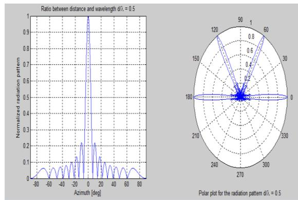
Figure 8: Radiation pattern when array element is 16 while the separation distance is  $0.5\lambda$
