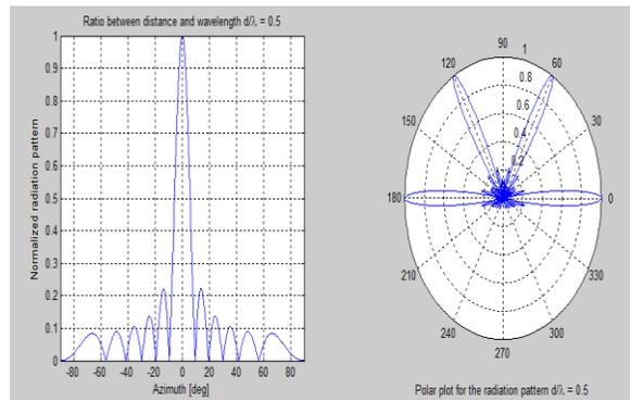
Figure 7: Radiation pattern when array element is 12 while the separation distance is  $0.5\lambda$
