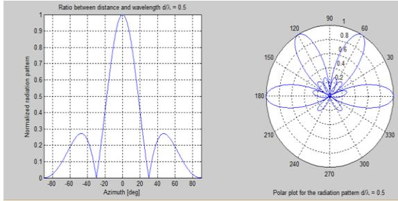
Figure 2: Plot of radiation pattern with 4 element array and separation distance  $0.5\lambda$
