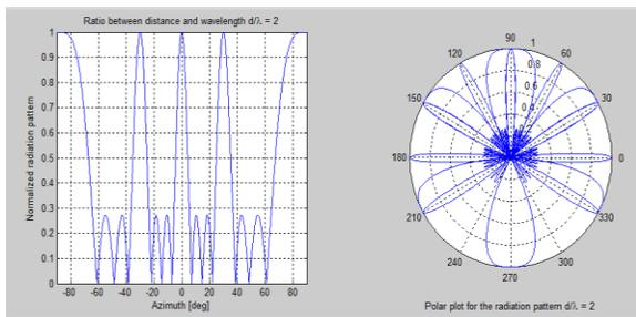
Figure 4: Plot of radiation pattern with 4 element array and separation distance  $2\lambda$
