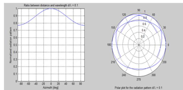
Figure 1: Plot of radiation pattern with 4 element array and separation distance 0.1 $\lambda$
