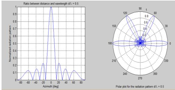
Figure 6: Radiation pattern when array element is 8 while the separation distance is  $0.5\lambda$
