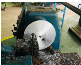
Figure 12. Shaping of Cutting Disc
