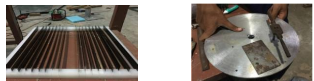
Figure 16. Rectangular Cutting Blade
