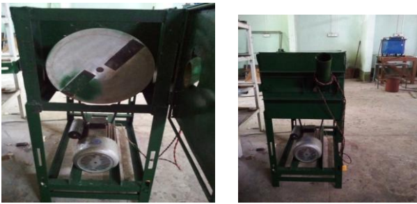
Figure 17. Front View with Cutting Disc and Inlet Hopper
