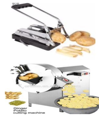
Figure 1. Manual and Automatic potato slicing machines
