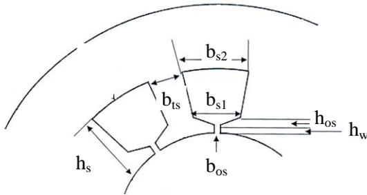
Fig.1. Main Dimension of Stator Slot and Core
