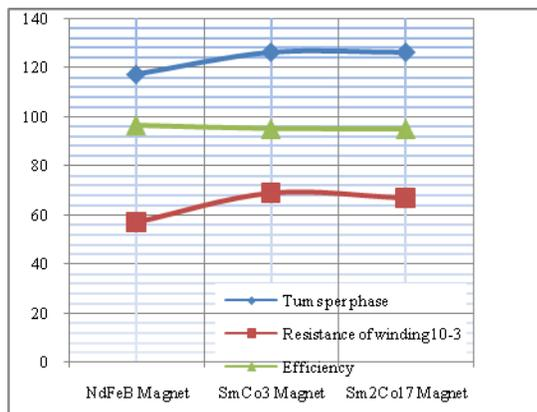
Fig.5. Permanent Magnet Synchronous Motor 50 kW Using NdFeB Magnet, SmCo<sub>3</sub> Magnet and Sm<sub>2</sub>Co<sub>17</sub> Magnet
