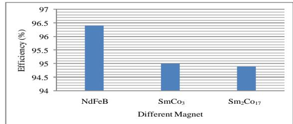
Fig.2. Efficiency of 50 kW PMSM for Different Magnet
