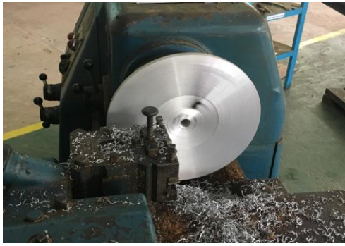
Figure.7 Reducing the Thickness of Cutting Blade in a Lathe
