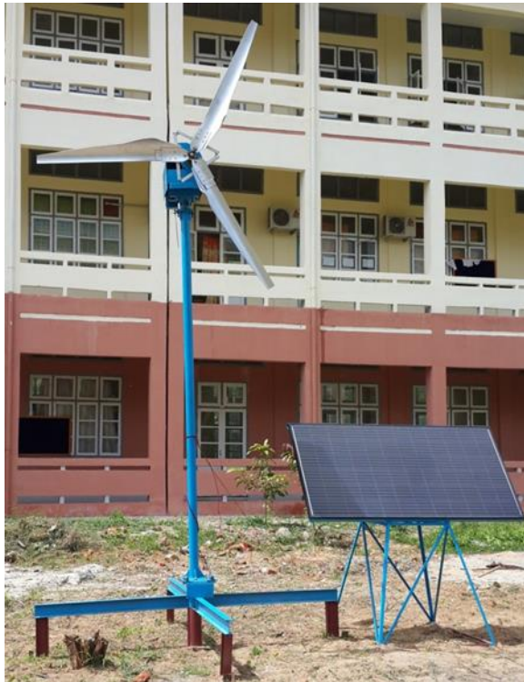
Fig 3. Wind Solar Hybrid System
