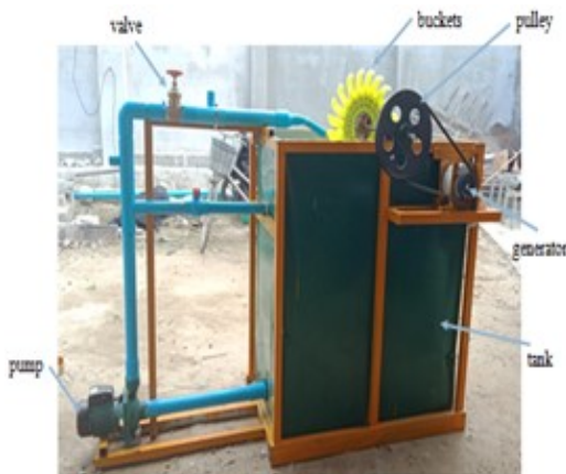
Fig. 4: Constructed Turgo Turbine
