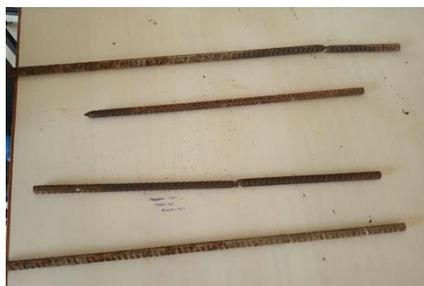
Fig 3(a) Failure of newly manufactured steel bars
