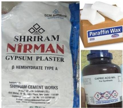
Fig.6.1 material used to make specimen
