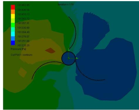
After the input data is ready, the model then is entering the meshing process. The meshing is viewed through a cut plot as shown in Figure. The fluid is experienced separation when it passes through the blade and this region is considered as high-gradient flow region. The mesh control is set to be finer in this region to obtain better solution accuracy.
