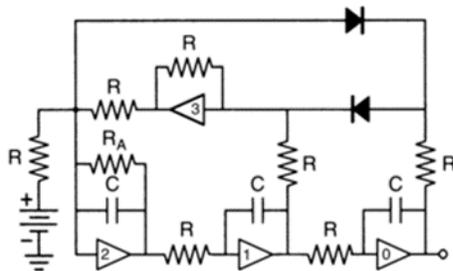
In the above circuit, all resistors are of equal value, except  $R_A=R/A=5R/3$ , and all capacitors are of equal size. The dominant frequency will be  $1/2\pi RC$ . The output of op amp 0 will correspond to the  $x$  variable, the output of 1 will correspond to the first derivative of  $x$  and the output of 2 will correspond to the second derivative.
