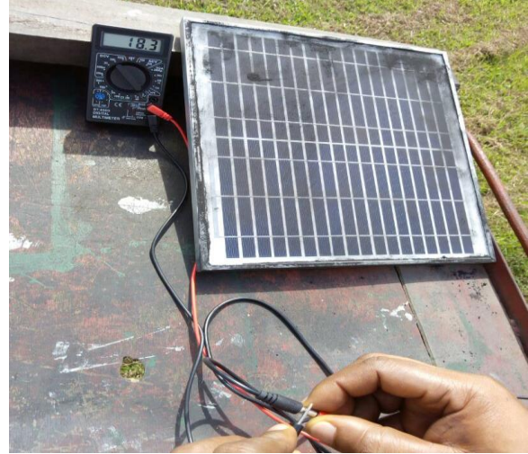
Figure 2: Experimental Setup for PV panel with soot
