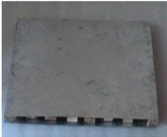
Fig. 6. Al skinned Bamboo truss core sandwich
