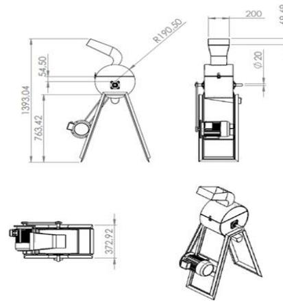
Figure 1: Orthographic Projection of the comminution equipment
