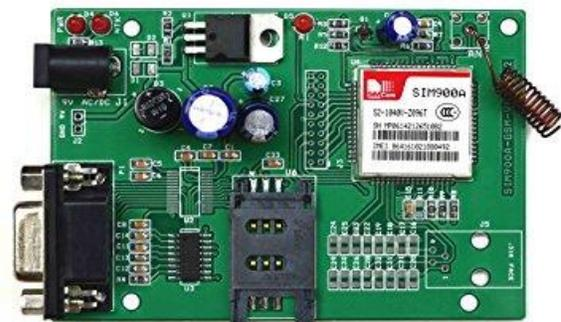
Figure 3. GSM Module
