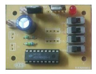
The RF receiver module that operates over 433Mhz is as follows:
