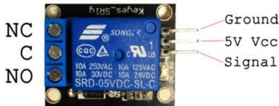
Figure 4: volts relay with pin description
