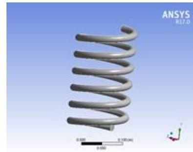
Fig 5. Geometry Model of Coil Spring for Modal Analysis
