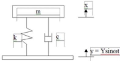
Fig. 3 . Single Degree of Freedom Model of a Vibration System with Viscous Damping
