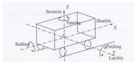
Figure 1. Quarter Car Suspension Model of 6 DOF
