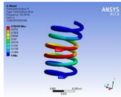
Fig 11. Natural Frequency of Mode Shape Four for Coil Spring
