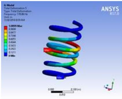
Fig 12 Natural Frequency of Mode Shape Five for Coil Spring
