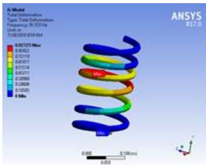
Fig 8. Natural Frequency of Mode Shape One for Coil Spring
