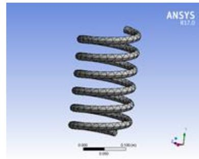
Fig 6. Meshed Model of Coil Spring for Modal Analysis
