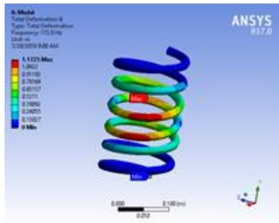
Fig 13. Natural Frequency of Mode Shape Six for Coil Spring
