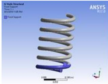
Fig 7 Boundary Condition of Coil Spring for Modal Analysis
