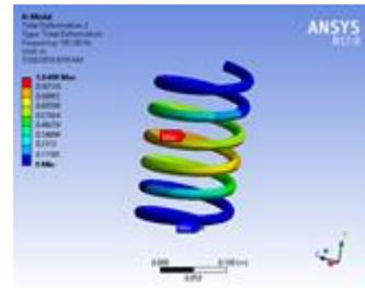
Fig 9. Natural Frequency of Mode Shape Two for Coil Spring
