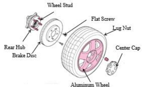
Fig 2. Aluminium Wheel is fastened to the Rear Hub with Steel Studs and Lug Nuts [16]
