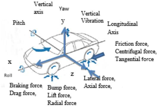
Fig 3. Forces Acting on the Car [1]
