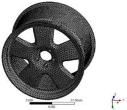
Fig 5. Meshing of Wheel's Rim
