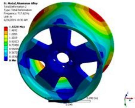
Fig 7. Second Mode Shape of Wheel's Rim
