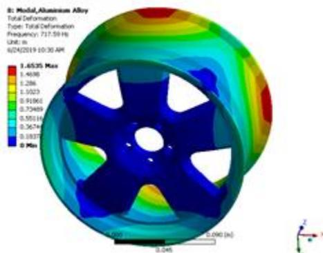
Fig 6. First Mode Shape of Wheel's Rim
