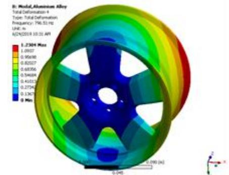
Fig 9. Fourth Mode Shape of Wheel's Rim
