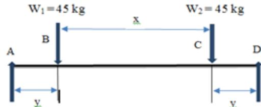
Figure 8. Load acting on the shaft of the trolley
