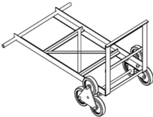
Figure 12. Isometric view of stair climbing trolley
