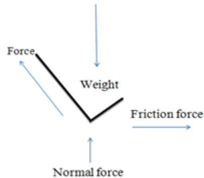
Figure 7. Force acting on the trolley
