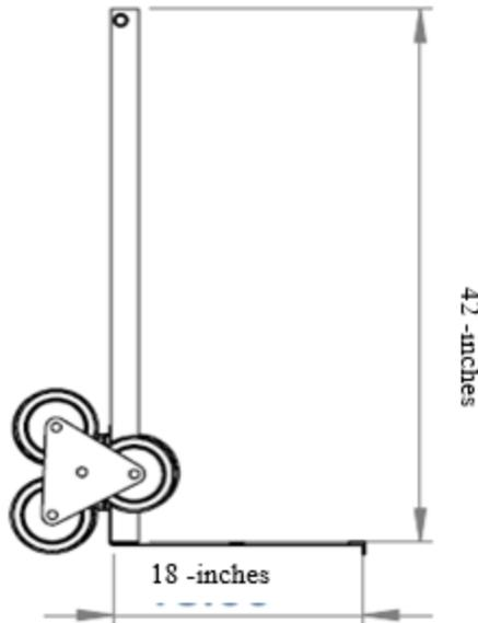
Figure 11. Modelling of side view of trolley
