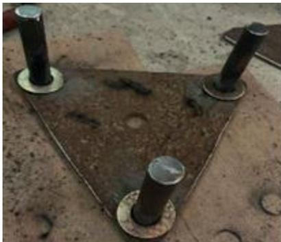
Figure 5. Fitting the tri-star plate with shafts
