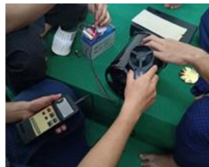
Figure 10. Measuring the velocity of air with anemometer
