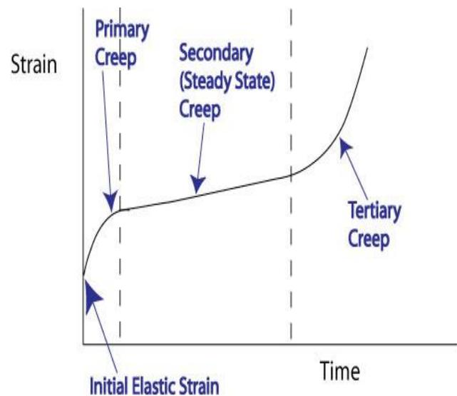
Fig 1: Creep Strain vs. Time Curve
