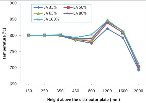
Fig. 2: Temperature variation along combustor axial height for CS combustion
