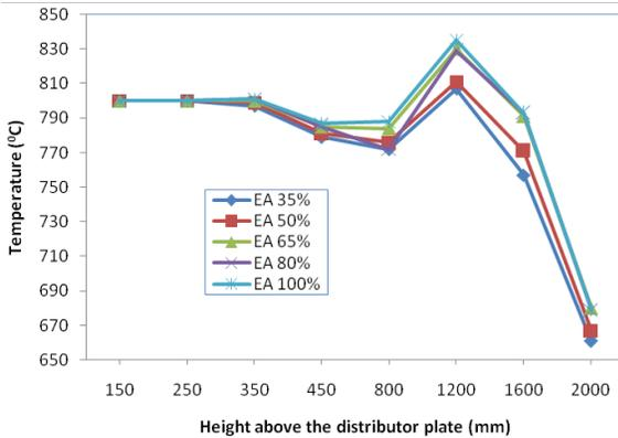
Fig. 3: Temperature variation along combustor axial height for RH combustion
