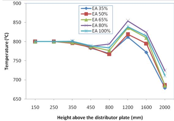
Fig. 5: Temperature variation along combustor axial height for GH combustion
