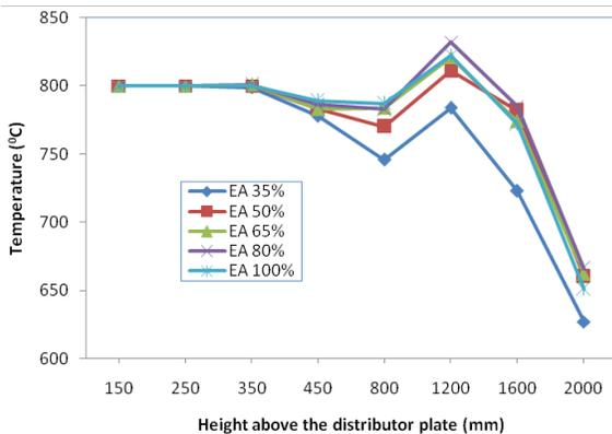
Fig. 4: Temperature variation along combustor axial height for CC combustion
