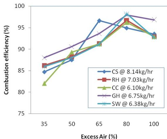
Fig. 9: Combustion efficiency for the various biomass fuels combustion at various percentage excess air
