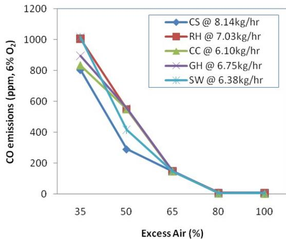
Fig. 7: CO emissions at 6% O<sub>2</sub> in flue gases for the various biomass fuels combustion
