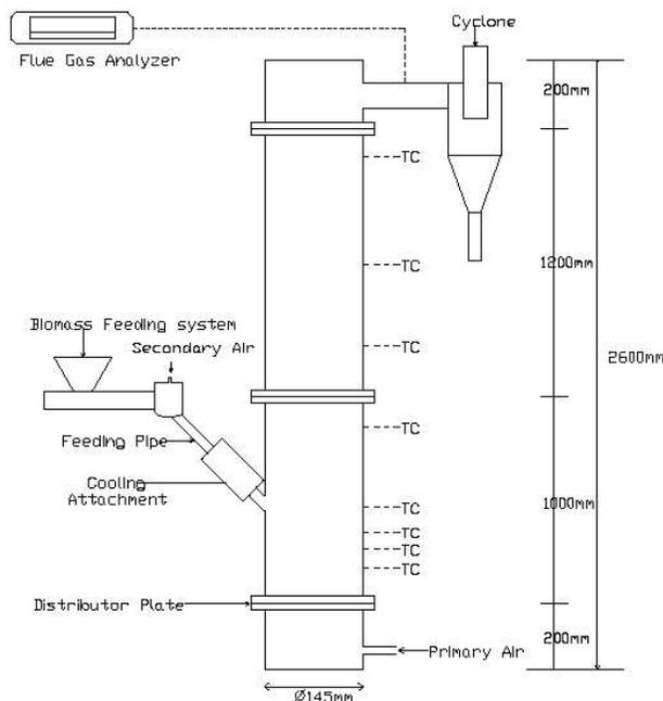
Fig. 1: Schematic diagram of the fluidized bed combustor
