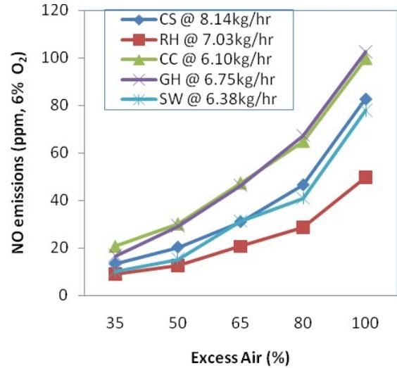
Fig. 8: NO emissions at 6% O<sub>2</sub> in flue gases for the various biomass fuels combustion
