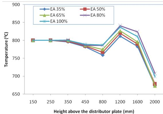
Fig. 6: Temperature variation along combustor axial height for SW combustion
