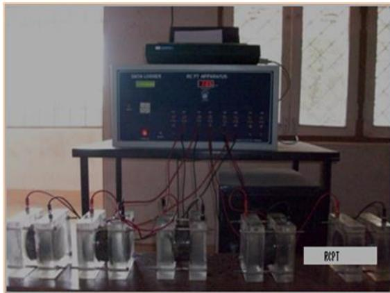
Figure 7: Experimental arrangement of RCPT
