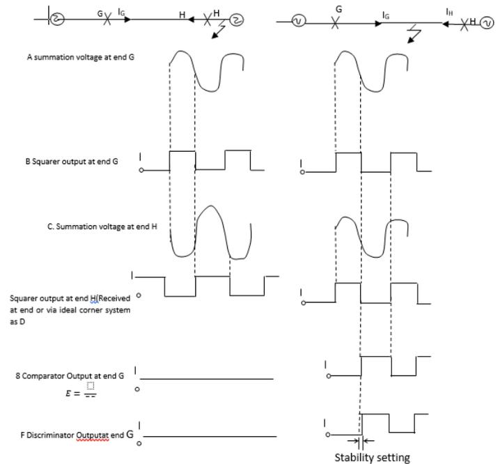
Fig. 2: Principles of phase comparison protection:(a) block diagram (b) output signals
