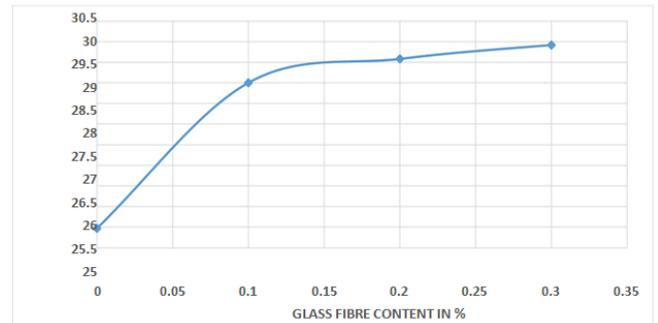
**Split Tensile Strength of Concrete (in N/mm<sup>2</sup>)**
