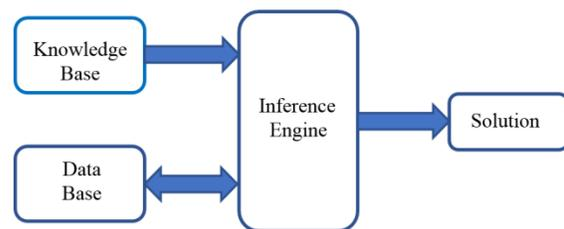
Fig. 2.1: Simplified block diagram of an XPS
