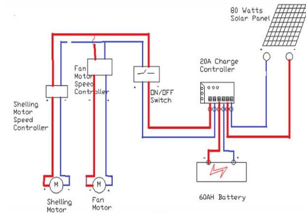
Figure 2: Electrical Photovoltaic – Appliances Interface
