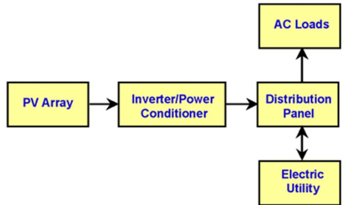
b. Diagram of grid-connected photovoltaic system
