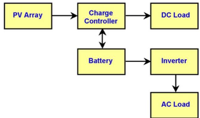
c. Diagram of stand-alone PV system with battery storage powering DC and AC loads
