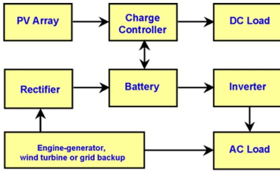
d. Diagram of photovoltaic hybrid system
