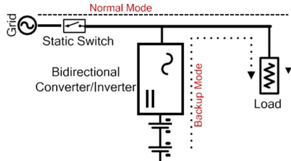
Fig. 2: - Block Diagram of Line Interactive UPS system.
