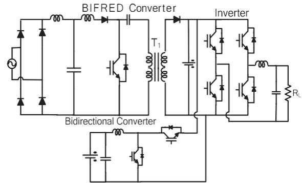
Fig. 3: - UPS system with BIFRED Converter
