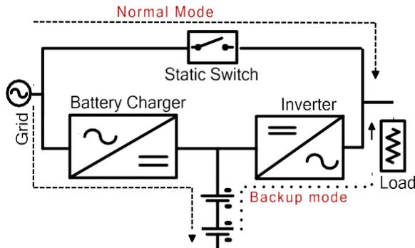
Fig. 1: - Block Diagram of Offline UPS System.
