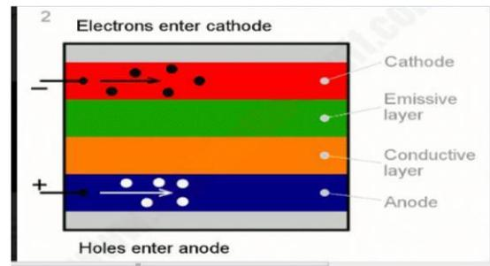
Fig. 2: - Entering of holes and electrons
