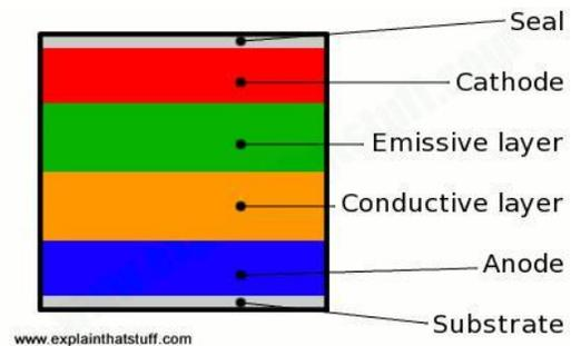
Fig. 1: - Layers of Diode
