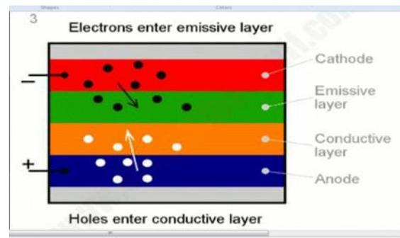
Fig. 3: - Transferring of holes and electrons
