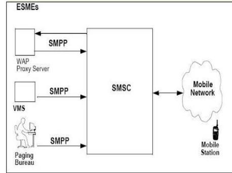
SMPP: SMPP is an open, industry standard protocol designed to provide a flexible data communications interface for the transfer of short message data between External Short Message Entities (ESME), Routing Entities (RE) and Message Centers. A Message Centre (MC) is a generic term used to describe systems such as a Short Message Service Centre (SMSC), GSM Unstructured Supplementary Services Data (USSD) Server, or Cell Broadcast Centre (CBC).
