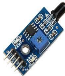
Fig -1: Flame Detecting Sensor
