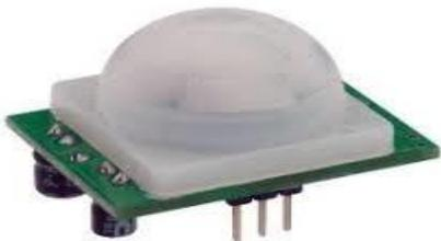
Fig.4. PIR Motion Sensor
