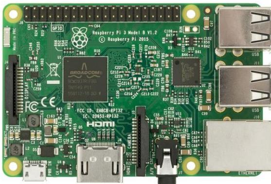
The Raspberry Pi 3 uses a Broadcom BCM2835 processor which is developed as the System on Chip (SoC) Technology. There have been various versions of the Raspberry Pi hardware advancing itself for every succeeding version.
