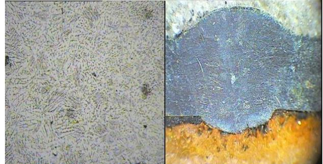
Fig 4. Grain Structure of SS 3041 (Etched With Aqua Regia 3:1 Hno3: Hcl) & Weld Picture
