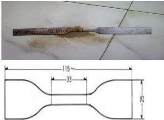
Fig 3 Specimen for Tensile Test According ASME SEC IX / 2007 Standard
