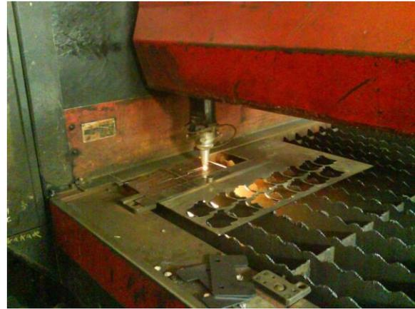
Figure1: CO2 Laser cutting operation
