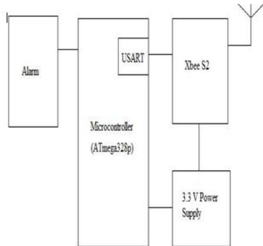
Figure 2: Receiving Part of wireless earthquake
