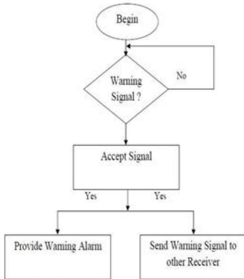
Figure 5: Receiving part work flow
