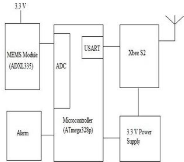
Figure 1: Transmitting part of wireless earthquake alarm system
