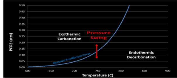
Fig 2: Reaction fully reversed - Pressure swing
