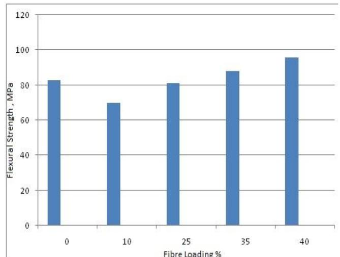
Figure 4. Flexural strength v/s Fibre Loading %
