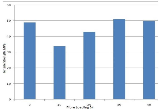
Figure 3. Tensile strength v/s Fibre Loading %
