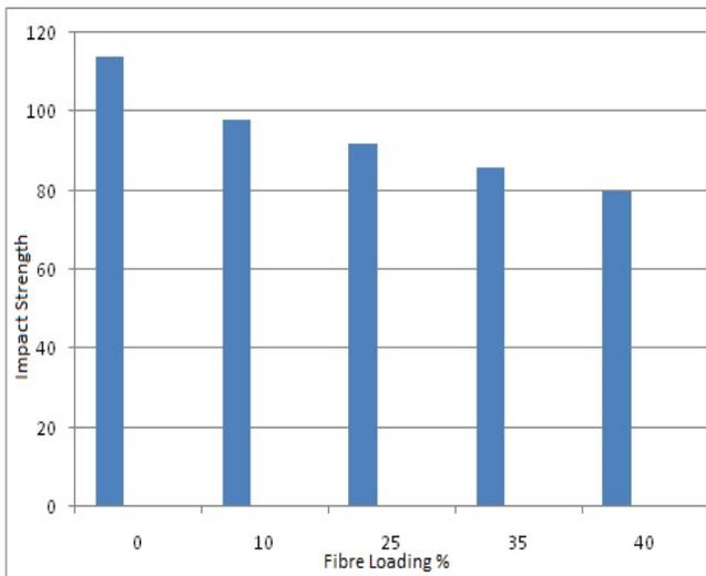
Figure 5. Impact strength v/s Fibre Loading %
