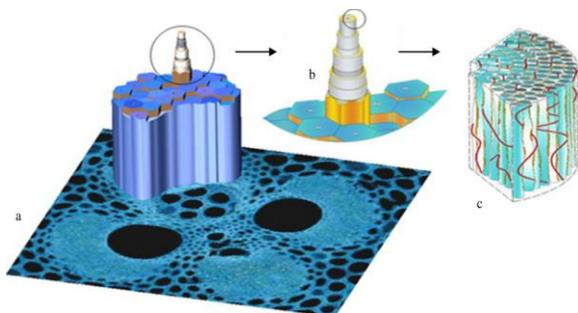
Fig.3. (a) Vascular bundle of bamboo, (b) elementary fiber 10–20  $\mu\text{m}$ , (c) Nano fibril 1–10  $\mu\text{m}$  involves lignin and hemicellulose [08].
