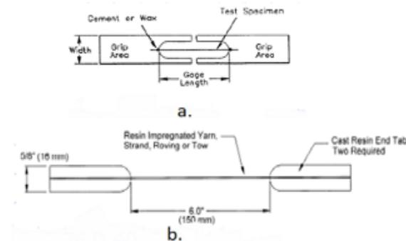
Figure 9: (a) Fiber testing, (b) Tow testing. [43]
